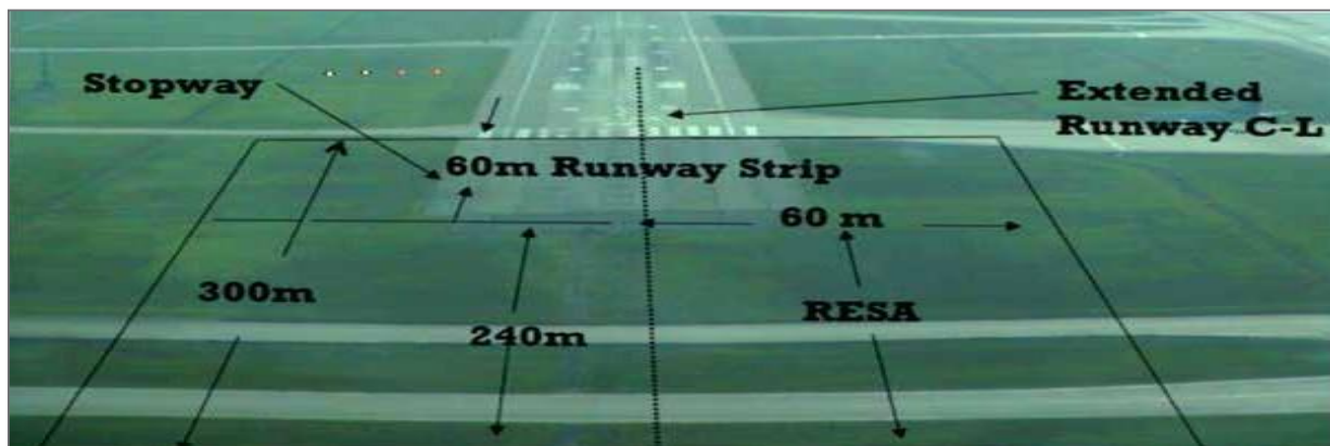
Figure 6. Depicted Runway End Safety Area showing recommended dimensions for a code 3 and 4 runway
